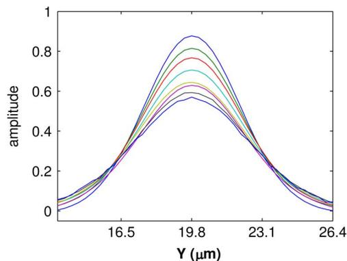
Fig. 4. Amplitude of the OPC refocused light pulse for various thicknesses of the scattering medium. The top to bottom curve corresponds to a scattering medium with thickness of 40, 80, 120, 160, 200, 240, 280, and 320  $\mu\text{m}$ , respectively.
