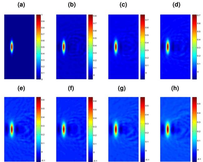
Fig. 3. OPC refocused light pulse of various thicknesses of scattering medium. The initial incident light pulse with a FWHM of  $9.3 \mu\text{m}$  is shown in (a). The thickness of the scattering medium is varied between  $80$  and  $320 \mu\text{m}$ . (b)  $80 \mu\text{m}$ , (c)  $120 \mu\text{m}$ , (d)  $160 \mu\text{m}$ , (e)  $200 \mu\text{m}$ , (f)  $240 \mu\text{m}$ , (g)  $280 \mu\text{m}$ , and (h)  $320 \mu\text{m}$ , respectively.
