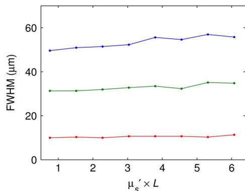
Fig. 5. Cross-sectional width of the OPC refocused light. Incident light of three different cross-sectional widths are shown (bottom to top): 9.32, 29.97, and 47.3  $\mu\text{m}$ . The FWHM for various incident light pulses are plotted versus transport mean free path ( $\mu'_s \times L$ ). [ $L$ : thickness of the scattering medium;  $\mu'_s$ : reduced scattering coefficient corresponding to wavelength  $\lambda = 1 \mu\text{m}$ ].
