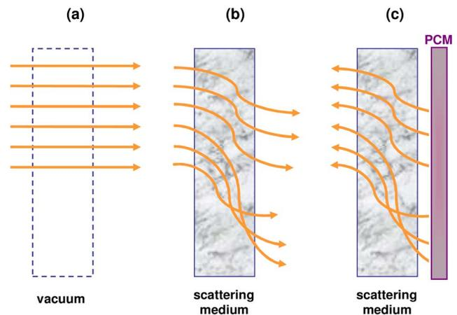
Fig. 1. Schematic of optical paths distorted by the presence of a scattering medium and refocused by a phase conjugate mirror (PCM). (a) Uniform incident light propagates straight through vacuum. (b) Optical paths of uniform incident light distorted by the scattering medium. (c) After incident upon PCM, the OPC effect causes light to propagate in reversed directions.
