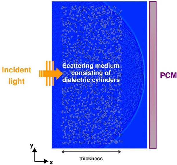
Fig. 2. 2-D PSTD simulation of the OPC phenomenon. Incident light undergoes multiple scattering as it propagates through scattering media. After incident upon a PCM, the OPC phenomenon causes light to propagate in reversed directions, back-trace its previous optical path, and return to where it originated.
