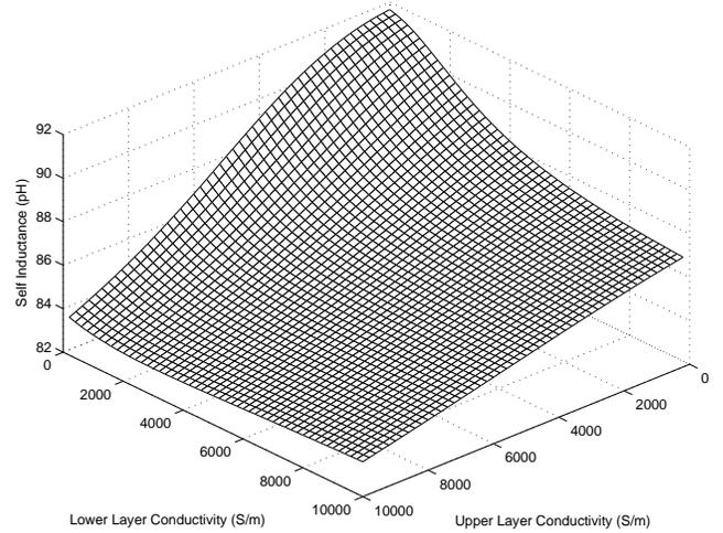
Fig. 9. With the same conductivity, the upper layer substrate will have larger effect than the lower layer. However, the lower layer cannot be ignored when the thickness of the upper layer is less than its skin depth.
