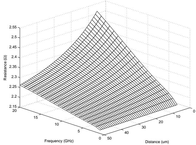
Fig. 8. Resistance increases as frequency increases and conductor-substrate distance decreases.
