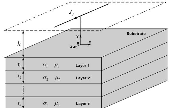
Fig. 1. A current filament parallel to a multilayer substrate which contains different layers of different thickness, conductivity, and permeability.
