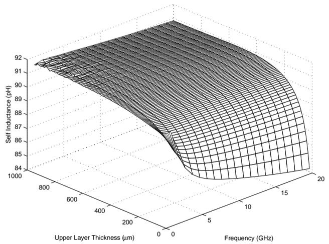
Fig. 10. Self inductance saturates when the thickness of the upper layer grows over its skin depth.
