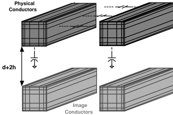
Fig. 2. Eddy-current-aware PEEC model. Each conductor is further discretized to consider the uneven distribution of currents.
