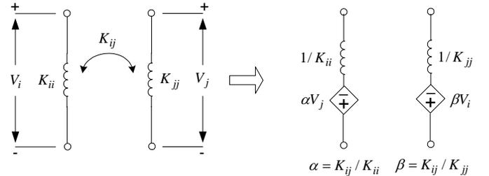
Fig. 4. SPICE compatible model for reluctance. The original reluctance element is substituted by serial self inductance and VCVSs.
