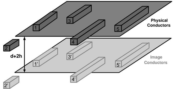
Fig. 3. Extended window selection algorithm to simultaneously consider physical and image conductors.
