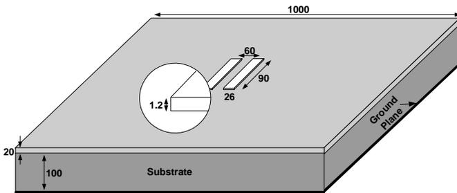
Fig. 5. Test configuration: two parallel copper interconnects above a two-layer substrate (Length unit:  $\mu m$ ).
