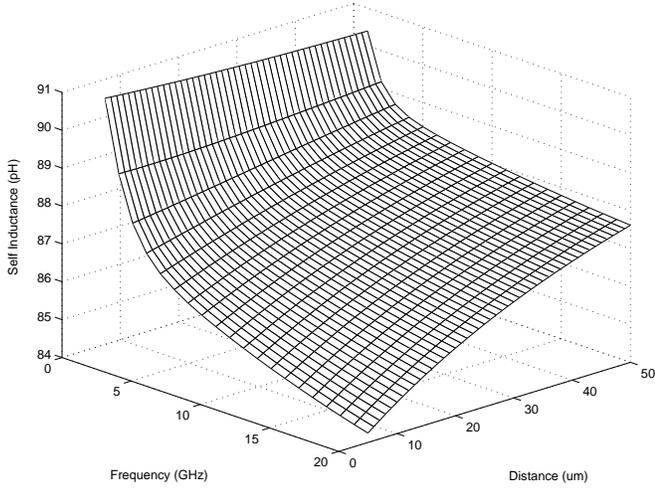
Fig. 7. Self inductance decreases as frequency increases and conductor-substrate distance decreases.
