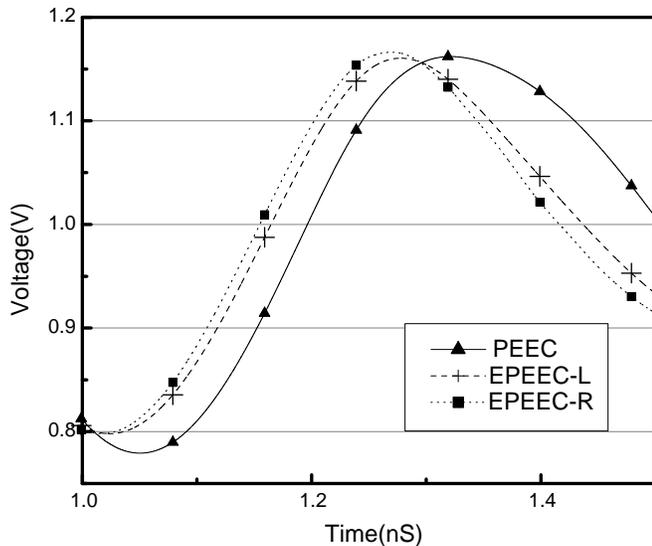
Fig. 11. Waveforms of transient responses by using different interconnect models: PEEC, EPEEC-L, and EPEEC-R.
