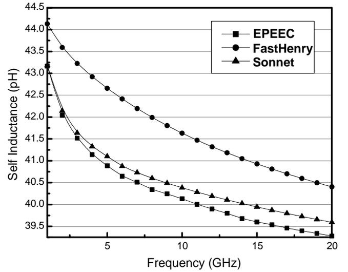
Fig. 6. Self inductance comparison by using three different extraction tools: FastHenry, Sonnet<sup>®</sup>, and EPEEC.
