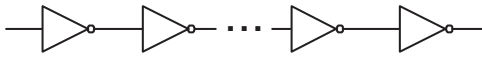
Figure 1. Circuit with linear structure has timing complexity O[N^2] since no small local sensitivity terms can be lumped
