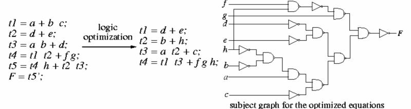
Methods/CAD tools: The Quine-McCluskey method (exponential-time exact algorithm), Espresso (heuristics for two-level logic), MIS (heuristics for multi-level logic), Synopsys, etc.
